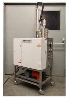
The NanoFeed system has been engineered for industrial or development use. It delivers a stable, pulse-free suspension stream, to achieve repeatable, high quality coatings.
